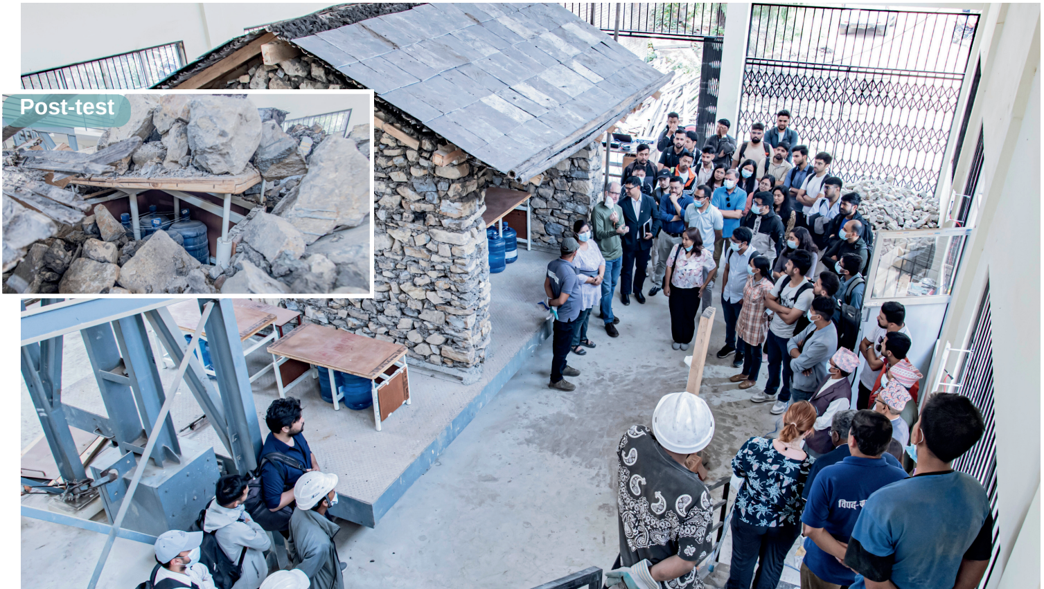
Nepal-made Earthquake Desks tested on a "shock table" with full-sized stone masonry walls and slate roof. Results were exciting—desks held the protective area below. Nepal has a vast number of collapse-prone schools of stone masonry construction. Earthquake Desks provide an interim life-saving solution to protect students until communities can replace or strengthen their existing buildings.
